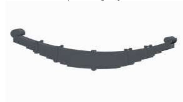
Fig.1 CAD model of parabolic leaf spring
